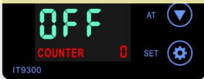
Heat press enters into power off mode if machine is kept quietly for set time and without any operation
