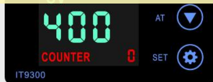
User can wake up heat press and start heating by touching any key
